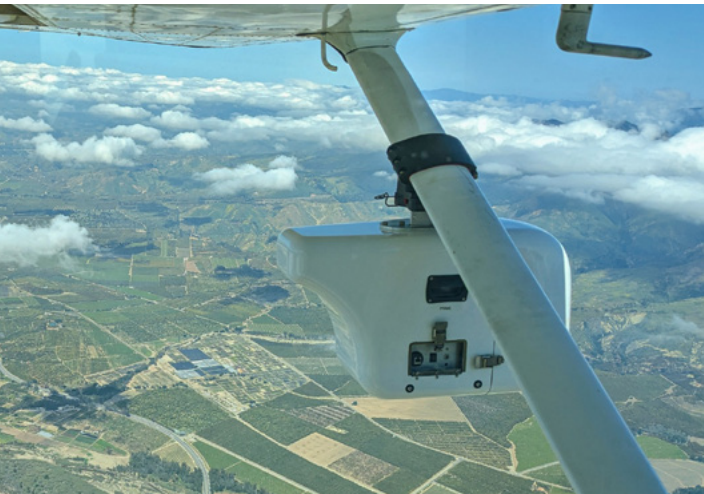
Methane Leak Detection via Aerial Flyover. Source: Insight M.
